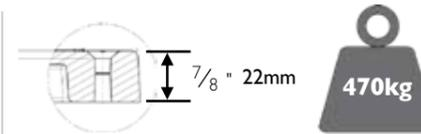
The N&C Premier Shower Deck is ideal for creating a level access wet floor area with ease. With a self supporting structure, Premier Shower Deck can be placed directly onto underfloor joists without the need for additional support. The built-in falls in the deck encourage the swift removal of waste water.
