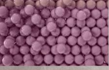
Micro granules used in Nicobond Grouts
