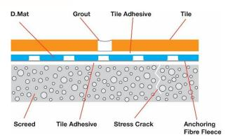
The cut lengths of the D-Mat 3L will be butt jointed (placed edge to edge) and these joints covered with Nicobond Jointing Tape or similar self adhesive reinforcing tape.
